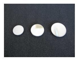
Mark & model : IP25, The diameter of mirror is 25mm and basic material is Si. The product is plated with multi-layer dielectric film, which enjoys cleaning durability and the reflecting rate is about 99.85%.
